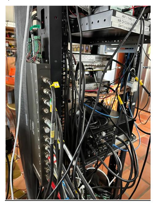
Attach antenna coaxes that were plugged into the remote station antenna switch to the 3x11 antenna switchbox on the floor. The positions should correspond to the positions on the display box with the LEDs. Here is the common setup:
